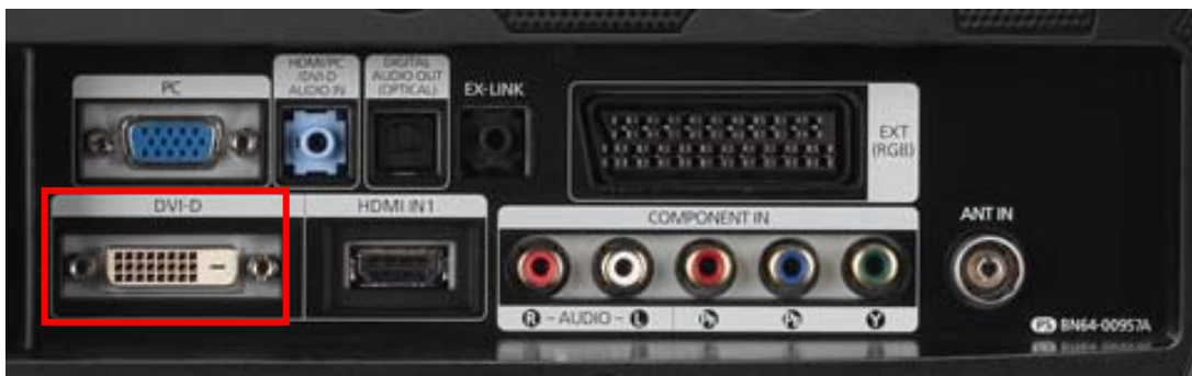
Figure 5 DVI-D Connector TFT detail example
