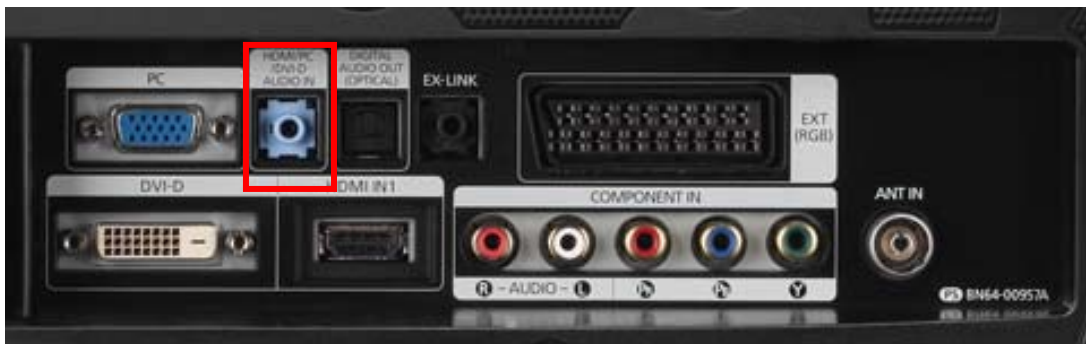
Figure 8 Stereo input Connector TFT detail example
