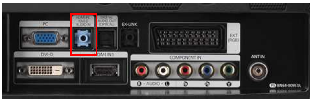
Figure 8 Stereo input Connector TFT detail example
