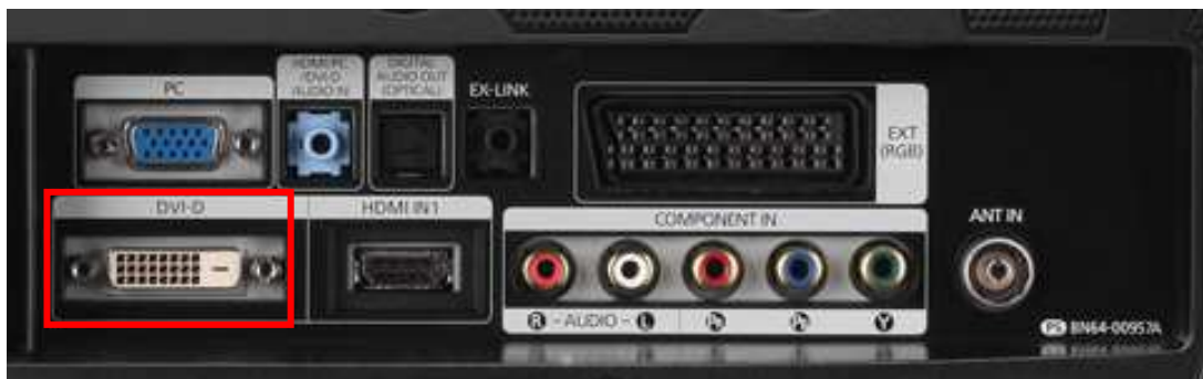
Figure 5 DVI-D Connector TFT detail example
