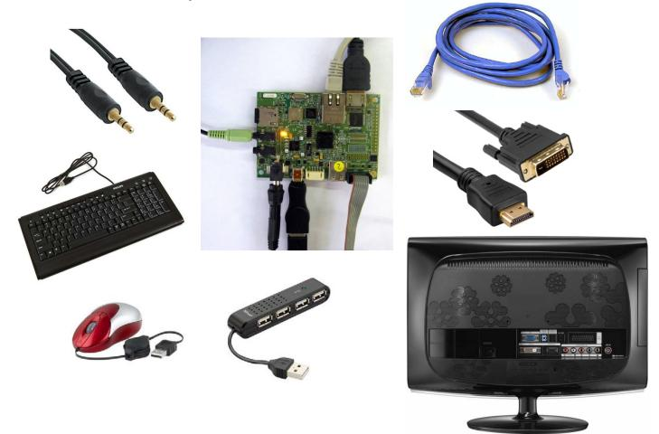
b. Before powering the IGEPv2 board, check that you have plugged in the DVI cable, the USB HUB, the USB keyboard and the USB mouse.
