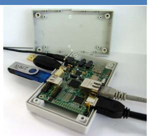
Wall mounting facility is provided in two ways, either by separately designed feet or by precut holes in the base.
